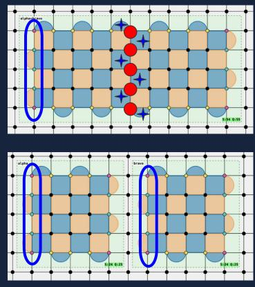
The old logical Z operator is redefined as logical Z operator of one the logical qubits. The logical Z operator of the other logical qubit is defined as the product of the logical Z operator of the first logical qubit and the measured values of the Z stabilizers (marked in figure).
