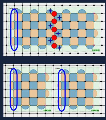
Take note that regardless of the logical state encoded by the old logical qubit, the logical state of the new logical qubits post-Split will be stabilized by logical ZZ, given by the product of the marked Z-stabilizers.
