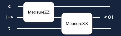
The logical CNOT can be implemented through measurement of Pauli operators, as depicted in the above figure, up to single-qubit Pauli corrections on both control and target qubits.
