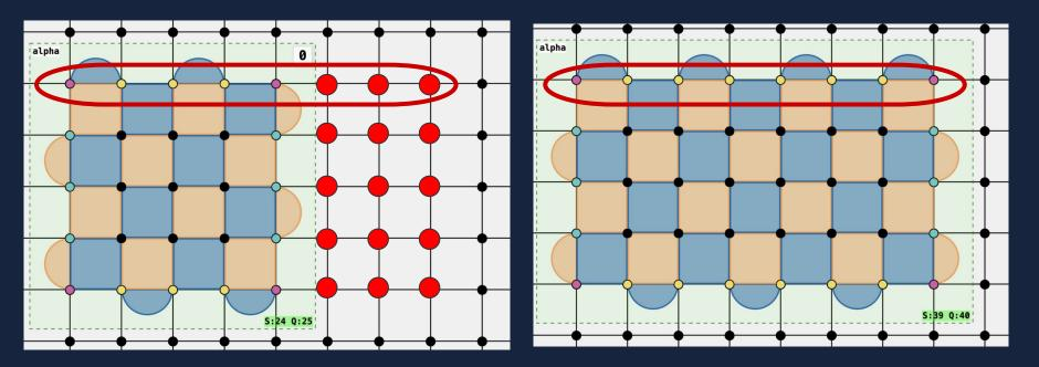
Prior to Grow (extending in the X-logical direction), data qubits to be included into the new patch are set to +X state.
