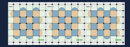
Start by preparing the single "long" patch, initialized in the +X logical state. Then perform the Split operation, breaking up the existing logical X operator into 3 individual ones.
