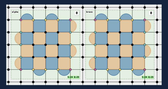
Selecting a set of data qubits in Entwine that includes boundaries of 2 adjacent patches creates the Merge operation.
