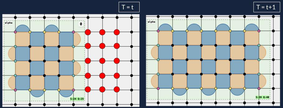
At any particular time step, some physical qubits are part of a logical qubits and some are not. By altering these sets based on a set of well-defined rules, we can build a sequence of such time-steps that **alter the shapes, orientation, and size of these logical qubits**.
