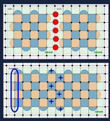
Just like the previous Split operation, the new logical qubit post-Merge is stabilized by the product of the marked Z-stabilizers, equivalent to the logical ZZ operator of the old logical qubits.
