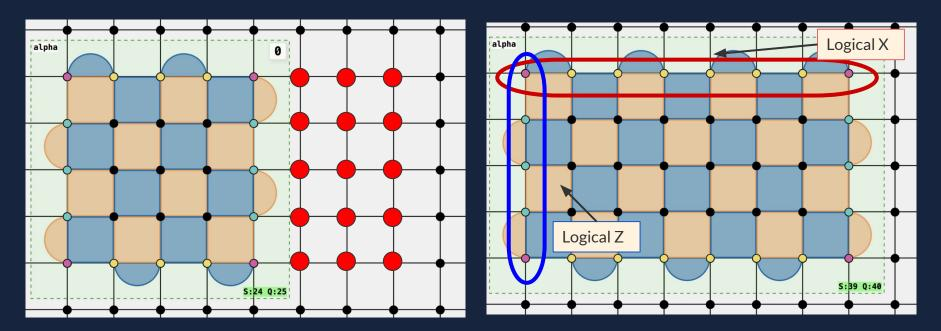
A logical qubit (of the surface code) refers a collection of physical qubits where syndrome-measuring circuits "enforce" a set of stabilizers from the surface code,
