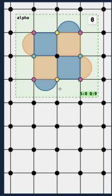
Likewise, prior to Grow (extending in the Z-logical direction), data qubits to be included into the new patch are set to +Z state. Logical X is unchanged, while logical Z is similarly changed as in the previous example.
