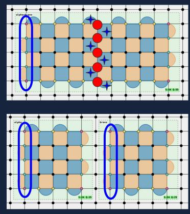
Because the eigenvalue of the logical ZZ operator is known (determined), the Split operation is also a part of the logical Measurement operation of Pauli ZZ.
