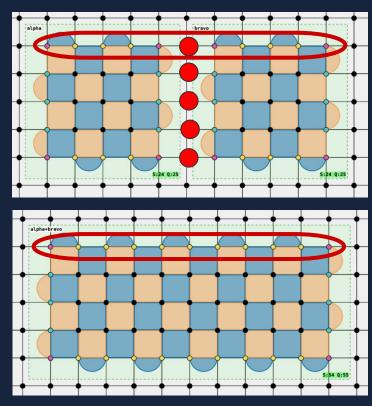
The Merge on the X boundary lines up the 2 separate logical X operators of their respective logical qubits, to create a single new logical X operator.
