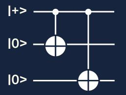
To implement this circuit with surface code logical qubits, we need to consider how to implement the logical operations such as CNOT with lattice surgery.
