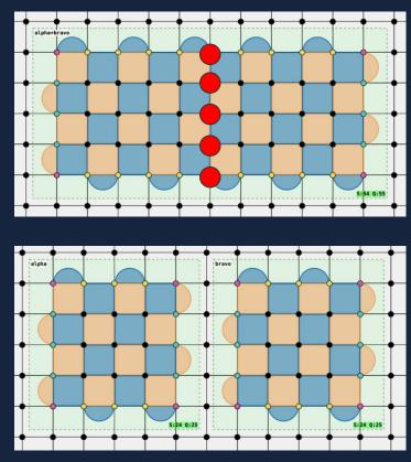
A subset of data qubits that were part of the old logical qubit is measured out in the X basis, in such a way as to result in 2 logical qubits after.
