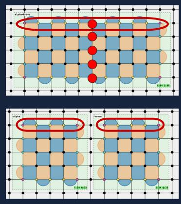
The old logical X operator is related to the new logical XX operator, with the product of one the data qubits that was measured. The eigenvalue of the the new logical XX operator is influenced by the measured value of the data qubit.
