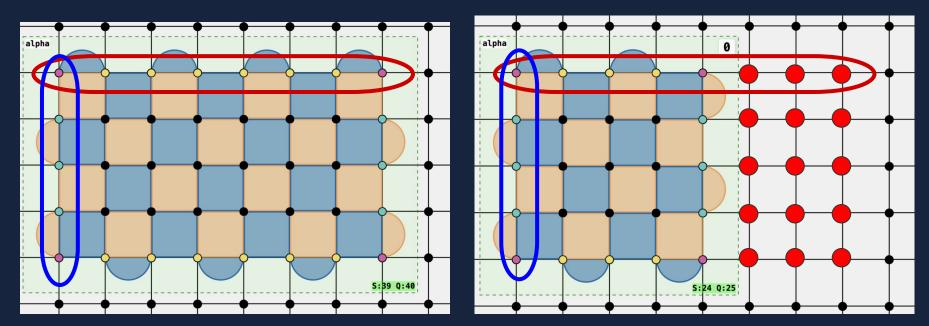
The new logical X operator is related to the old logical X operator by the product of the measurement values of the data qubits that were part of the old logical X but no longer part of the new one.
